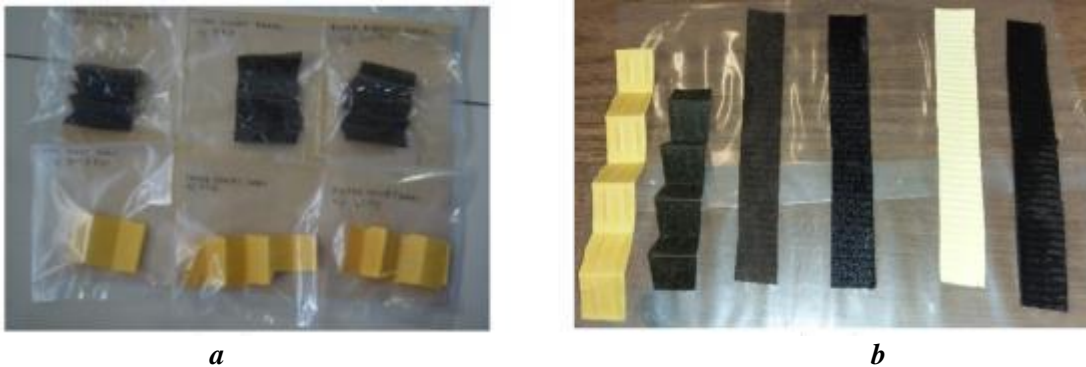
Fig. 2. Pieces of filter paper for analysis: a) For SEM/EDS & FTIR and b) for GC
